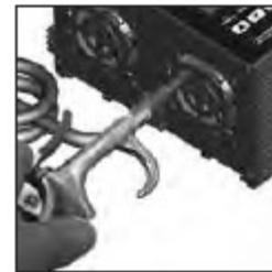
**12.4** Ensure that all of the charger components are in place and in good working condition, including the plastic boots on the battery clips.
