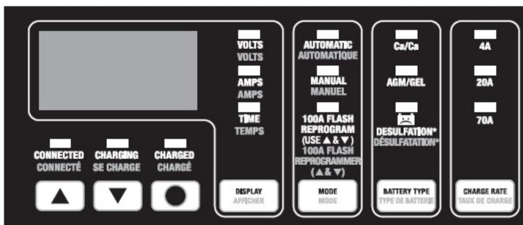
**CONNECTED (yellow/orange) LED** The CONNECTED LED will light when the battery is properly connected.
